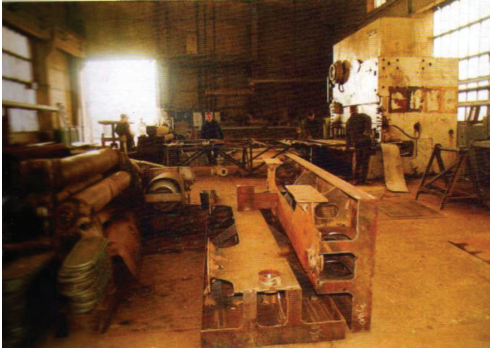
Hardware shop (former shop of rotary iron cleaning). Production of trash racks for Nijegorodskaya hydroelectric power plant
