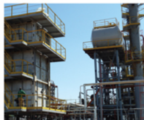
Platforms with equipment and rectification columns made from stainless steel and titanium
